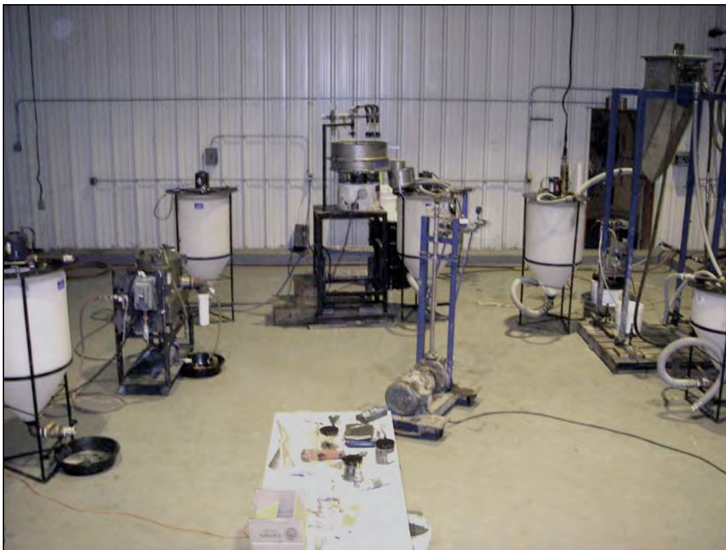
Photo 3 – Pump Skid, Centrifuge, Shaker Screen, and Collision Chamber
